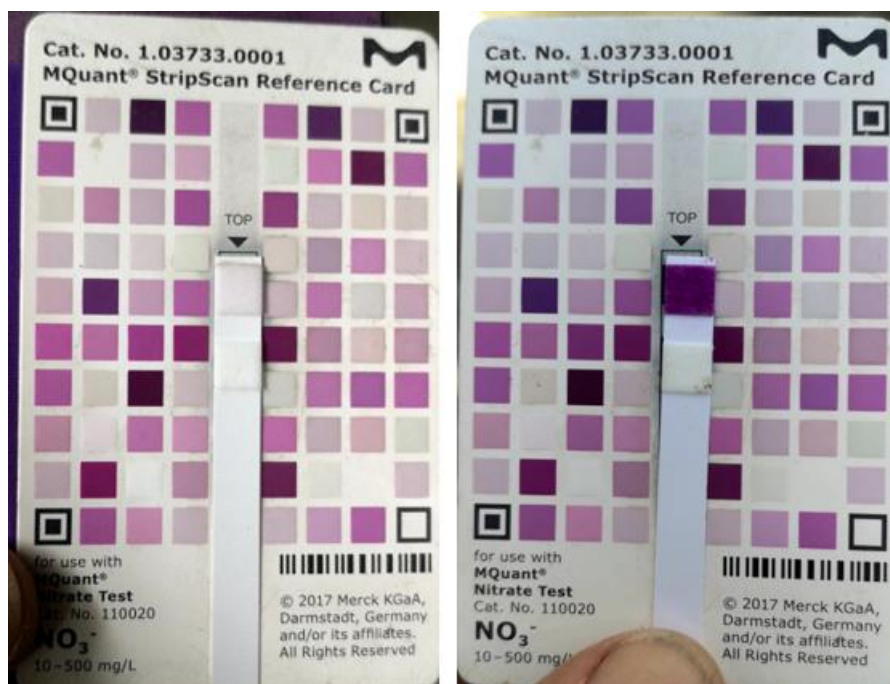
Figure 1 MQuant StripScan Reference Cards showing very low (left) and high (right) nitrate concentrations from solution prepared from soil samples. A phone app is used to capture the image and determine concentration based on colour comparisons.
